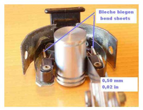
Adjusting the points has to be approved with sense, power and skillfulness. I used flat-nose-pliers and after some trying out got exact adjustments.
